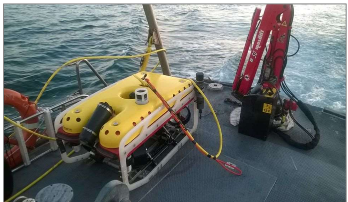
Figura 24 –ROV (Remotely Operated Vehicle)
