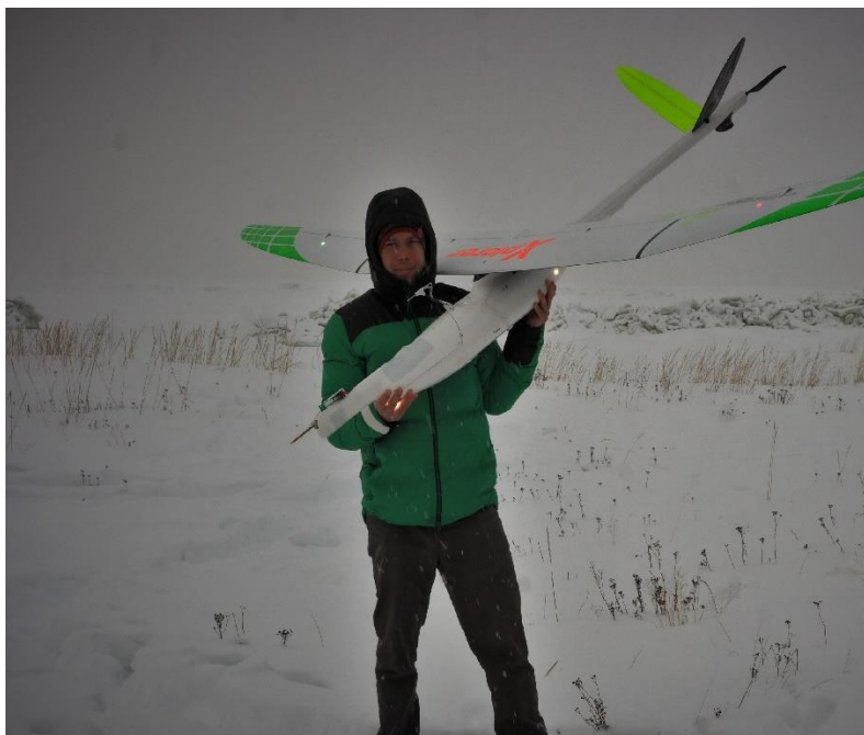
Fig. 11.126: il drone ad ala fissa MASC-3 ( Multi-Purpose Airborne Sensor Carrier ; Kral 2020)
