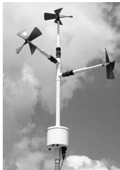
Fig. 11.19: propeller triassiale Gill UVW (R.M. YOUNG Company)
